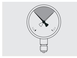
The pressure gauge should be installed in such a way as to avoid exposure to heat and vibration and to enable the dial indication to be easily read.
